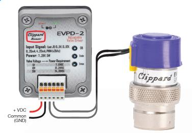
The EVPD proportional valve driver fast-tracks valve control applications. This product is ideal for laboratories and OEM product development and can be customized to fit OEM applications including control parameters. The EVPD produces driver current for Clippard's EVP or DVP series valves proportional to input control signals.
