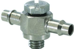
Minimatic barb fittings provide a flexible, easy alternative to ferrule and push-to-connect/push-quick fittings. Designed for use with urethane hose, barb fittings will provide a leak-free connection that will hold well beyond the working pressure of the hose without the need for additional clamps.
