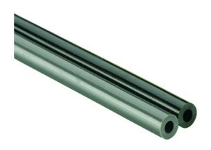
Flexible, durable 1/8" I.D. vinyl plastic hose, but two hoses molded together, one side has rib the entire length for identification. Ideal for feeding supply in on one line and out on the other, reduces labor, makes neat assembly and may be parted with any sharp edge.
