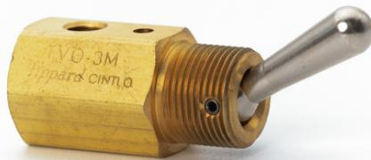
The function of a 2-Way valve is to turn an air supply on and off. In the "on" position, medium flows from the inlet to the outlet, and in the "off" position, the flow is blocked. 3-Way styles have an exhaust port which vents the outlet to the atmosphere. Available with #10-32 and 1/8" NPT ports.
