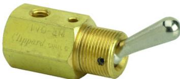
The function of a 2-Way valve is to turn an air supply on and off. In the "on" position, medium flows from the inlet to the outlet, and in the "off" position, the flow is blocked. 3-Way styles have an exhaust port which vents the outlet to the atmosphere. Available with #10-32 and 1/8" NPT ports.
