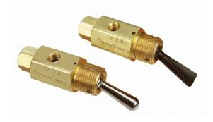
The function of a 2-Way valve is to turn an air supply on and off. In the "on" position, medium flows from the inlet to the outlet, and in the "off" position, the flow is blocked. 3-Way styles have an exhaust port which vents the outlet to the atmosphere. Available with #10-32 and 1/8" NPT ports.
