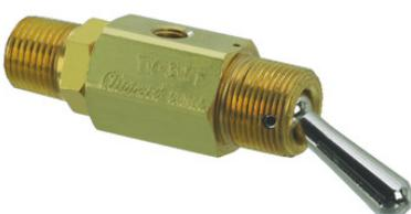
The function of a 2-Way valve is to turn an air supply on and off. In the "on" position, medium flows from the inlet to the outlet, and in the "off" position, the flow is blocked. 3-Way styles have an exhaust port which vents the outlet to the atmosphere. Available with #10-32 and 1/8" NPT ports.
