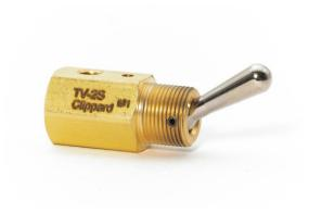
The function of a 2-Way valve is to turn an air supply on and off. In the "on" position, medium flows from the inlet to the outlet, and in the "off" position, the flow is blocked. 3-Way styles have an exhaust port which vents the outlet to the atmosphere. Available with #10-32 and 1/8" NPT ports.
