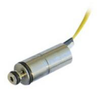
These 2-Way and 3-Way direct actuating valves offer an extremely fast response time for accurate dosing of minute volumes with the same long life you expect from the original Clippard EV line of electronic valves, in a 7 mm cartridge package. Due to very low moving weights, they are extremely quiet and emit very low vibration. Subminiature size and low energy consumption make them ideal for transportable and mobile systems, among others.
