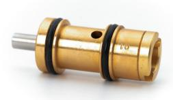
Cartridge valves are used to connect to air passages in manifolds or other valve circuit systems, thereby eliminating the need for external plumbing. Saves space and reduces the possibility of leaks.
