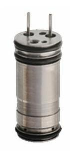
These 8 mm 3-Way direct actuating valves offer an extremely fast response time for accurate dosing of minute volumes with the same long life you expect from the original Clippard EV line of electronic valves, now in a 8 mm cartridge package. The valve was designed with a unique patented valving principle using Clippard's robust stainless steel "spider", with only one moving part that travels less than 0.007".
