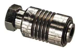
The J-Series sleeve valves with 1/8" NPT and 1/4" NPT ports offer large flow capability with a relatively short stroke in 2-Way and 3-Way valves, and no cross-over between inlet and exhaust on the 3-Way models.
