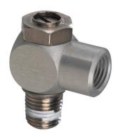
These combination needle and check valve flow controls are typically used to control air flow from air cylinders, thereby controlling the speed at which the piston strokes, either while extending or retracting, depending on their location in the circuit.
