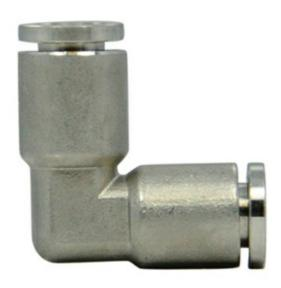
Constructed of high grade 316 stainless steel, these durable fittings provide a simple push-pull method of connecting pneumatic components to each other and system piping. Push-Quick fittings allow full flow through the hose/tubing I.D. with no smaller orifice required as in barb fittings.
