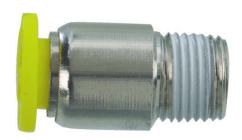
Clippard Push-Quick Fittings provide a simple method of connecting pneumatic components to each other and system piping. They are designed for use with both flexible hose and stiff tubing made of nylon, urethane, polyethylene or polypropylene.
