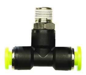
Clippard Push-Quick Fittings provide a simple method of connecting pneumatic components to each other and system piping. They are designed for use with both flexible hose and stiff tubing made of nylon, urethane, polyethylene or polypropylene.
