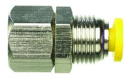
Push-Quick Fittings provide a simple method of connecting pneumatic components to each other and system piping. They are designed for use with both flexible hose and stiff tubing made of nylon, urethane, polyethylene or polypropylene.
