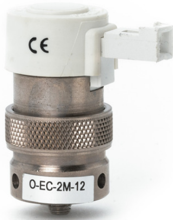
2-Way Elec. Valve, N-C, Manifold Mount, Pin Connector, 24 VDC, Oxygen
