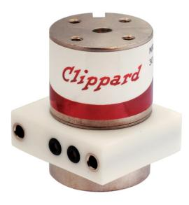
The NIV series media isolation valve is a solenoid-operated device that utilizes a flexible diaphragm to isolate the actuation mechanism from the fluid path. Media isolation valves are commonly used for a wide variety of applications, including those that require precise, repeatable dispensing of media for analytical instrumentation. All wetted areas of the valve are PTFE or PEEK, making this series ideal for use with corrosive media.
