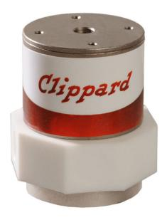
The NIV series media isolation valve is a solenoid-operated device that utilizes a flexible diaphragm to isolate the actuation mechanism from the fluid path. Media isolation valves are commonly used for a wide variety of applications, including those that require precise, repeatable dispensing of media for analytical instrumentation. All wetted areas of the valve are PTFE or PEEK, making this series ideal for use with corrosive media.
