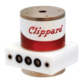
The NIV series media isolation valve is a solenoid-operated device that utilizes a flexible diaphragm to isolate the actuation mechanism from the fluid path. Media isolation valves are commonly used for a wide variety of applications, including those that require precise, repeatable dispensing of media for analytical instrumentation. All wetted areas of the valve are PTFE or PEEK, making this series ideal for use with corrosive media.
