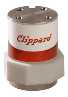
The NIV series media isolation valve is a solenoid-operated device that utilizes a flexible diaphragm to isolate the actuation mechanism from the fluid path. Media isolation valves are commonly used for a wide variety of applications, including those that require precise, repeatable dispensing of media for analytical instrumentation. All wetted areas of the valve are PTFE or PEEK, making this series ideal for use with corrosive media.
