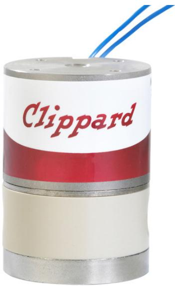
PIV series media isolation valves are solenoid-operated devices that utilize a flexible diaphragm to isolate the actuation mechanism from the fluid path. Media isolation valves are commonly used for a wide variety of applications, including those that require precise, repeatable dispensing of media for analytical instrumentation. All wetted areas of the valve are PEEK body and PTFE diaphragm, making this series ideal for use with corrosive media.
