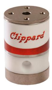
The NIV series media isolation valve is a solenoid-operated device that utilizes a flexible diaphragm to isolate the actuation mechanism from the fluid path. Media isolation valves are commonly used for a wide variety of applications, including those that require precise, repeatable dispensing of media for analytical instrumentation. All wetted areas of the valve are PTFE or PEEK, making this series ideal for use with corrosive media.
