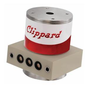
PIV series media isolation valves are solenoid-operated devices that utilize a flexible diaphragm to isolate the actuation mechanism from the fluid path. Media isolation valves are commonly used for a wide variety of applications, including those that require precise, repeatable dispensing of media for analytical instrumentation. All wetted areas of the valve are PEEK body and PTFE diaphragm, making this series ideal for use with corrosive media.
