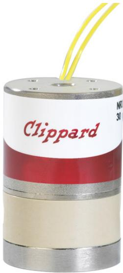
PIV series media isolation valves are solenoid-operated devices that utilize a flexible diaphragm to isolate the actuation mechanism from the fluid path. Media isolation valves are commonly used for a wide variety of applications, including those that require precise, repeatable dispensing of media for analytical instrumentation. All wetted areas of the valve are PEEK body and PTFE diaphragm, making this series ideal for use with corrosive media.
