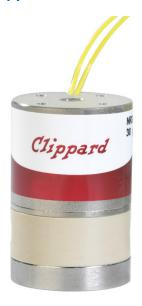
PIV series media isolation valves are solenoid-operated devices that utilize a flexible diaphragm to isolate the actuation mechanism from the fluid path. Media isolation valves are commonly used for a wide variety of applications, including those that require precise, repeatable dispensing of media for analytical instrumentation. All wetted areas of the valve are PEEK body and PTFE diaphragm, making this series ideal for use with corrosive media.
