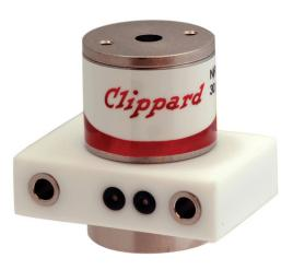
The NIV series media isolation valve is a solenoid-operated device that utilizes a flexible diaphragm to isolate the actuation mechanism from the fluid path. Media isolation valves are commonly used for a wide variety of applications, including those that require precise, repeatable dispensing of media for analytical instrumentation. All wetted areas of the valve are PTFE or PEEK, making this series ideal for use with corrosive media.
