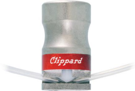
NPP Series 2-Way pneumatic pinch valves are air-piloted devices designed to open or close tubes for controlling flow of liquids and gases. Other valve types have internal passages that may cause small amounts of fluid to remain in the valve. Pinch valves have no areas or dead volume where fluid can become trapped. Only the inside of the tubing has contact with the fluid.
