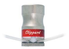
NPP Series 2-Way pneumatic pinch valves are air-piloted devices designed to open or close tubes for controlling flow of liquids and gases. Other valve types have internal passages that may cause small amounts of fluid to remain in the valve. Pinch valves have no areas or dead volume where fluid can become trapped. Only the inside of the tubing has contact with the fluid.
