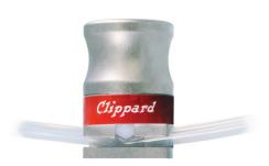
NPP Series 2-Way pneumatic pinch valves are air-piloted devices designed to open or close tubes for controlling flow of liquids and gases. Other valve types have internal passages that may cause small amounts of fluid to remain in the valve. Pinch valves have no areas or dead volume where fluid can become trapped. Only the inside of the tubing has contact with the fluid.
