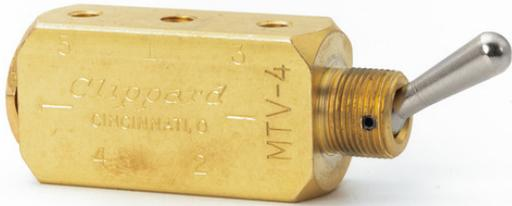
These #10-32 ported 2-Way, 3-Way and 4-Way valves are manually-actuated with a toggle. The toggles are NP steel and have a detent action. The MTV-5 has threaded exhaust and can be connected in a dual inlet pressure configuration.
