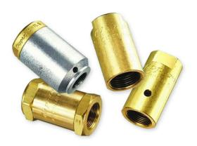
Air Pilot Valve Actuators thread onto the tops of Clippard miniature 2-Way, 3-Way, and 4-Way valves to provide fast pilot actuation from a pneumatic signal. They permit wide circuit flexibility and minimize cost, hazards and complexity by allowing many control functions to be accomplished pneumatically.
