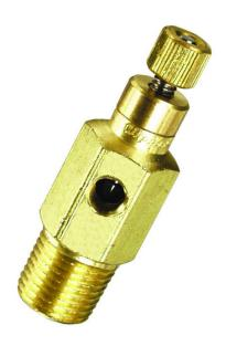
Adjustable control needle valves restrict flow in both directions. There are four models offered, all with #10-32 ports, but with various needle configurations to provide coarse or fine flow adjustment.
