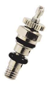
Adjustable control needle valves restrict flow in both directions. There are four models offered, all with #10-32 ports, but with various needle configurations to provide coarse or fine flow adjustment.
