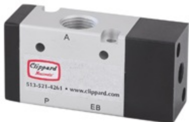
3/8" 3-Way Single Air Pilot Spring Return Valve
