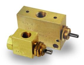
The MJV/MJVO series are high flow 1/8" NPT ported 2-Way, 3-Way and 4-Way valves that change their flow path when the stem is either depressed or released (spring return). The 2-Way and 3-Way valves are offered in both Normally-Closed and Normally-Open versions.
