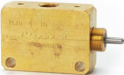
The MJV/MJVO series are high flow 1/8" NPT ported 2-Way, 3-Way and 4-Way valves that change their flow path when the stem is either depressed or released (spring return). The 2-Way and 3-Way valves are offered in both Normally-Closed and Normally-Open versions.
