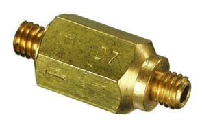
Check valves permit flow in one direction only. The MCV series is available with #10-32 ports and are construced of bright-dipped brass bodies that provide in-line mounting.
