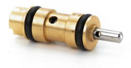
The MAV series are #10-32 ported valves that change their flow path when the stem is depressed or released. The 2-Way and 3-Way valves are offered in both Normally-Closed (not passing) or Normally-Open (passing) versions.
