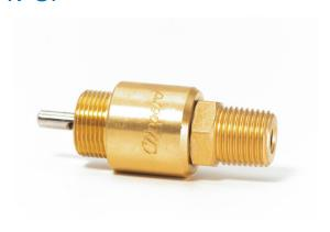
The MAV series are #10-32 ported valves that change their flow path when the stem is depressed or released. The 2-Way and 3-Way valves are offered in both Normally-Closed (not passing) or Normally-Open (passing) versions.
