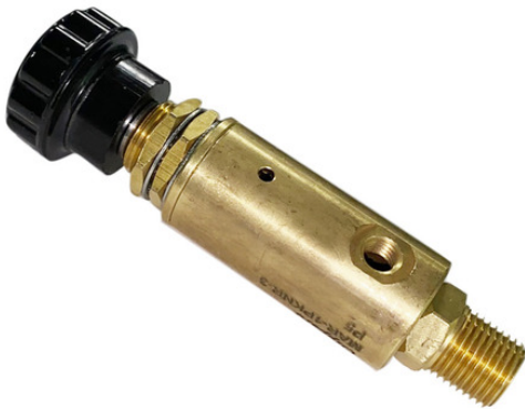
Pressure Regulator, 1/8" NPT-#10-32 Ports, Plastic Knob, 10-60 psig
