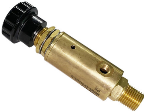
Pressure Regulator, 1/8" NPT-#10-32 Ports, Plastic Knob, 10-40 psig
