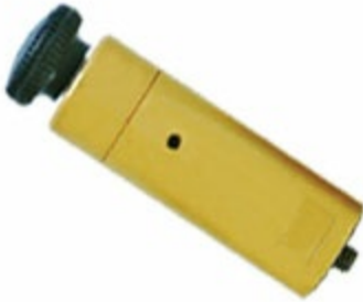
Pressure Regulator, #10-32 Mnfd. Mount, Non-Relieving, Plastic Knob, 10-60 psig
