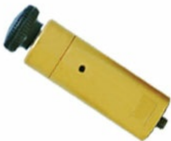
Pressure Regulator, #10-32 Mnfd. Mount, Non-Relieving, Plastic Knob, 10-70 psig
