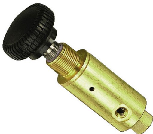
Pressure Regulator, #10-32 Ports, Plastic Knob, Non-Relieving, 10-30 psig
