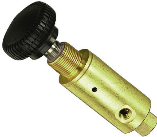
Pressure Regulator, #10-32 Ports, Plastic Knob, 10-50 psig
