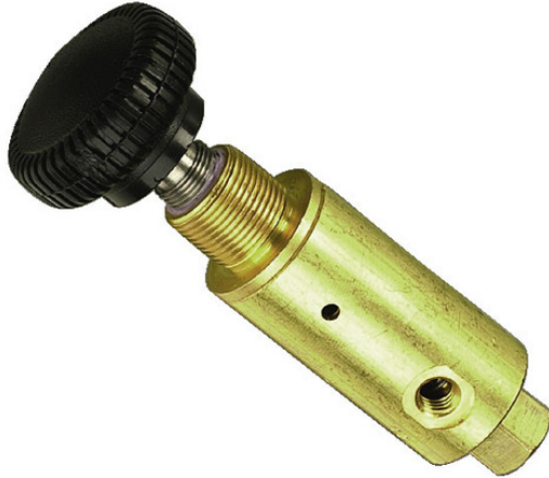
Pressure Regulator, #10-32 Ports, Plastic Knob, 10-20 psig
