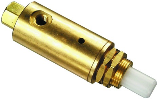
Pressure Regulator, #10-32 Ports, Plunger Actuated, 10-60 psig
