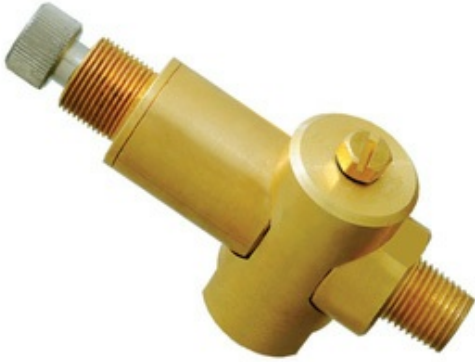
Pressure Regulator, 1/8" NPT Swivel Mount, Knurled Knob, Non-Relieving, 10-100 psig
